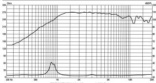
FREQUENCY (Hz), Measured-1W @ 1m
