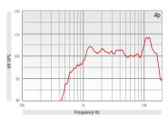
Frequency response curve of the horn measured on axis at distance of 1 meter with1 watt signal
