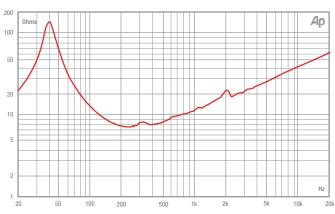
(3) Half space response measured in a 975 Litre sealed box. Blue line = fundamental 45° off-axis. Please note that the frequency response measurements are supplied for comparison only and are not a measure of the low frequency performance which may be achieved in a fully optimised system.
