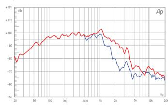
A.E.S. power handling test. Pink noise bandpass filtered at 12 dB per octave with cutoff frequencies of 40 Hz and
