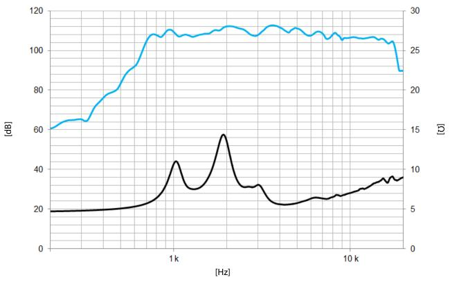
Note: On axis frequency response measured coupled to TD-164 horn in anechoic chamber, 1W / 1m
