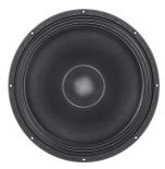
The 18PZW100\* is a long Xmax, high power subwoofer that features a triple roll surround. This proven model features a 21 mm long, 4 inch diameter (100mm) Copper wire voice coil. A 1000watt AES power rating, 97.6 dB sensitivity, and over 10.5mm of Xvar make the 18PZW100 an interesting alternative.
