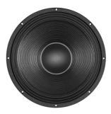
This next evolution subwoofer uses a new, longer, four layer aluminum voice coil. The result is less heat, more energy in the gap, higher sensitivity, higher power handling, lower distortion and better overall performance. The 18DS100 features a 36mm long, 4 inch diameter (100mm) Copper Clad Aluminum Wre voice coil. With a 1500watt AES power rating, 98 dB sensitivity, and over 14.0mm of Xvar, this high energy subwoofer is a significant step forward from similar models in the B&C range.
