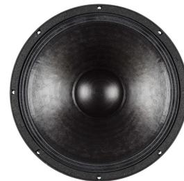
The NDL88 series is perfectly balanced for the loudspeaker systems of today. Incorporating a high temperature neodymium magnet inside the 3.5" (88mm) voice coil reduces the amount of steel needed in the motor structure, saving cost and weight. Unexpected low frequency output and midrange extension to meet with almost any driver for two way applications is the hallmark of this new performance-oriented woofer line from B&C Speakers. Do more, with less, with the NDL88 series.
