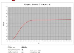
m SPL at 1 meter (dB): 118,3 equal to 698,6 Watts (Bass Band Power Rating)
